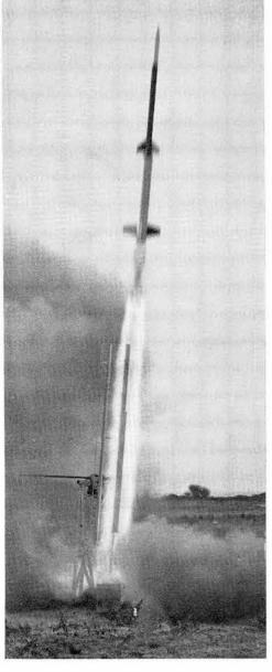
BLASTOFF—The slender Nitehawk 9 is fired on one of the 48 successful flights conducted to date. The Sandia-designed rocket system has carried a variety of instruments to altitudes of 175 to 200 miles.
